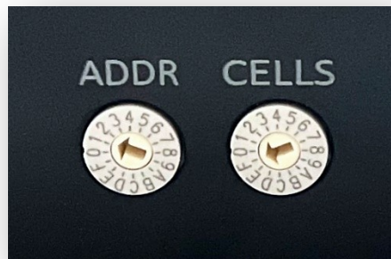
Figure 5: BMS address and cell selection rotary switches.
